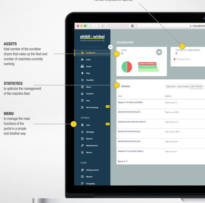
THANKS TO THE INTERCONNECTION BETWEEN THE DEVICE AND THE G&W FLEET 4 YOU CONNECT IT IS POSSIBLE TO VIEW THE STATUS OF THE MACHINE (E.G. WORKING HOURS, BATTERY ANALYSIS, COLLISIONS OCCURRED, ETC.) AND SCHEDULE MAINTENANCE ACTIVITIES
